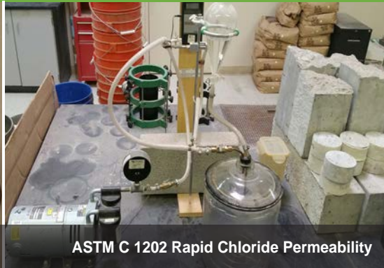
ASTM C 1202 Rapid Chloride Permeability
